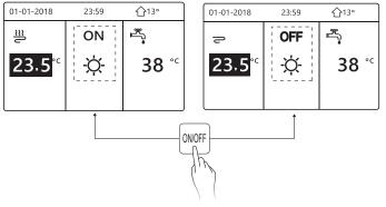
Use the room thermostat to turn on or off the unit for space heating or cooling.
